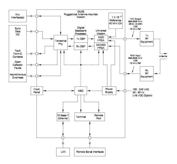
Figure 4-3. OM20 Outdoor Modem Functional Block Diagram
