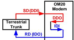
Figure 3-10. Insert Only with Eternal Frame Source
