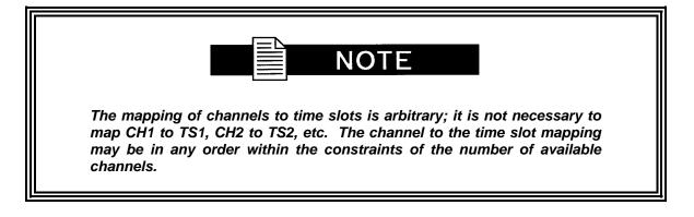
For example, ROM Map 1 could be used as the template for as Active Transmit (Drop) Map for a modulator configured for 64 Kbps operation. Only the first time slot of the T1 or E1 frame would be dropped into the modulator transmit path. The Drop Multiplexer would know to look only at the first entry in the Active Transmit table and would ignore the other 29 entries. If the map contained an "8" in its first entry, the eighth channel of the T1/E1 frame would be sent to the modulator.
