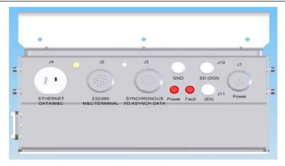
Figure 5-1. OM20 Front panel ports
