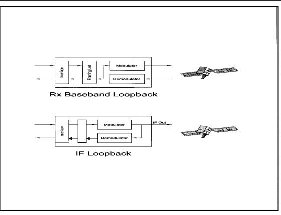
Figure 4-5. Loopback Functional Block Diagram
