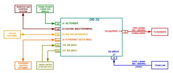
Figure 2-3. Outdoor Modem (OM) Interconnect Diagram
