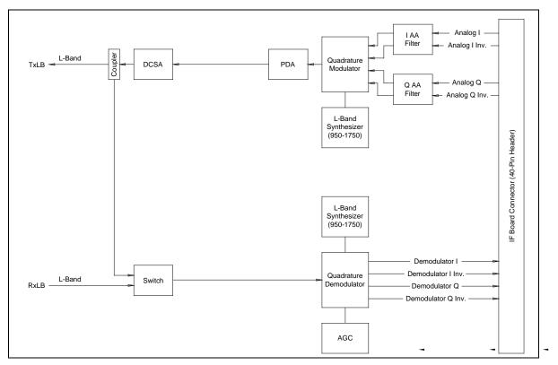
Figure 4-2. L-Band Card Block Diagram
