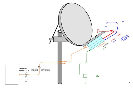
Figure 2-7. OM20 Feed Arm Mount, Ethernet Interface
