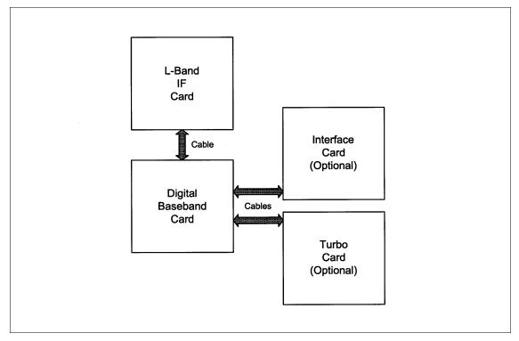
Figure 4-1. OM20 Block Diagram
