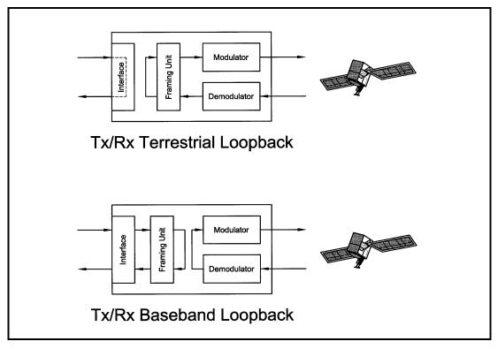
Figure 4-6. Loopback Functional Block Diagram
