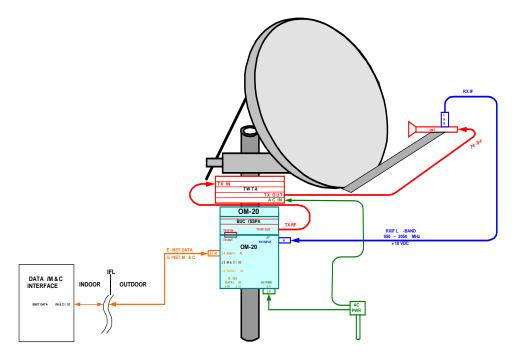
Figure 2-8. OM20 with High Power Amplifier, Ethernet Interface
