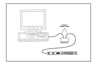
**Figure 1. Ethernet Connection**
