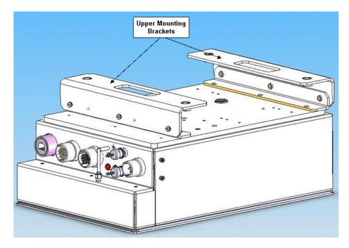
Figure 2.4. OM20 Mounting Brackets
